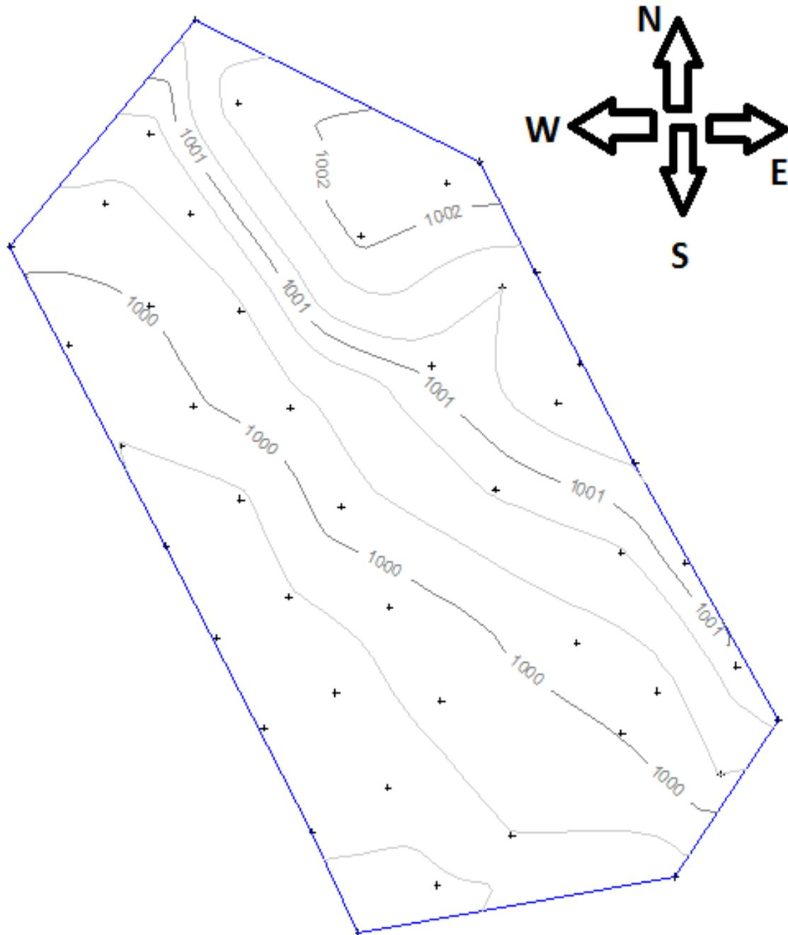
Figure D1 - Elevation Change Topography for Soccer Field
