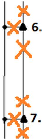
Figure 4 - Design 1: Exterior Loop Detail. Triangles indicate sprinkler heads, circles indicate connectors, and xs indicate shut-off valves.
