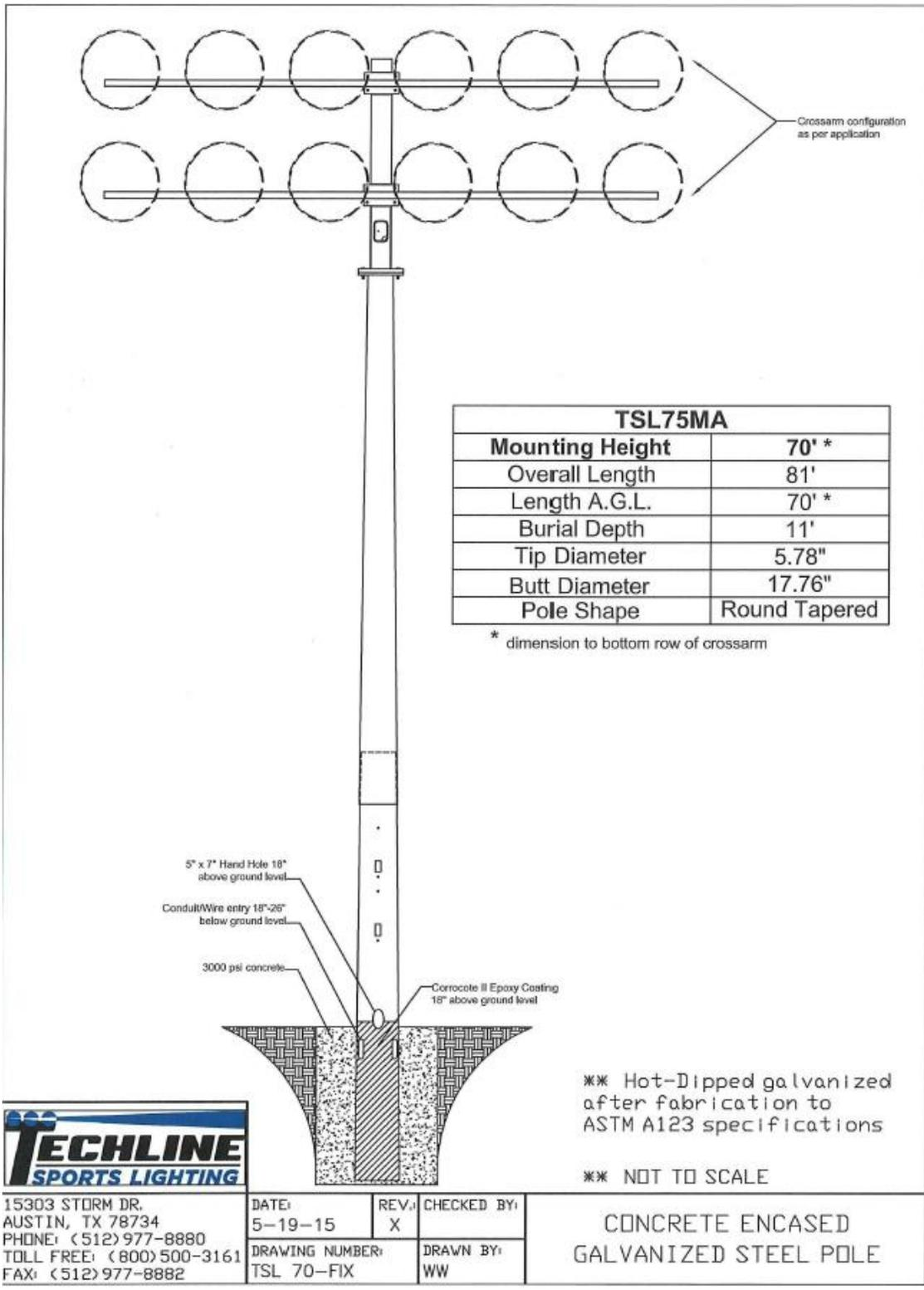
Figure B2 – Pole Design and Specs
