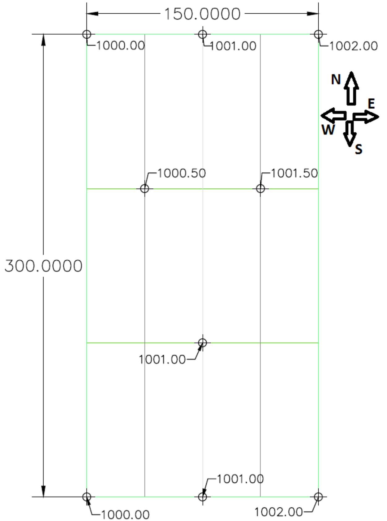
Figure 3 - Final elevation for soccer field location
