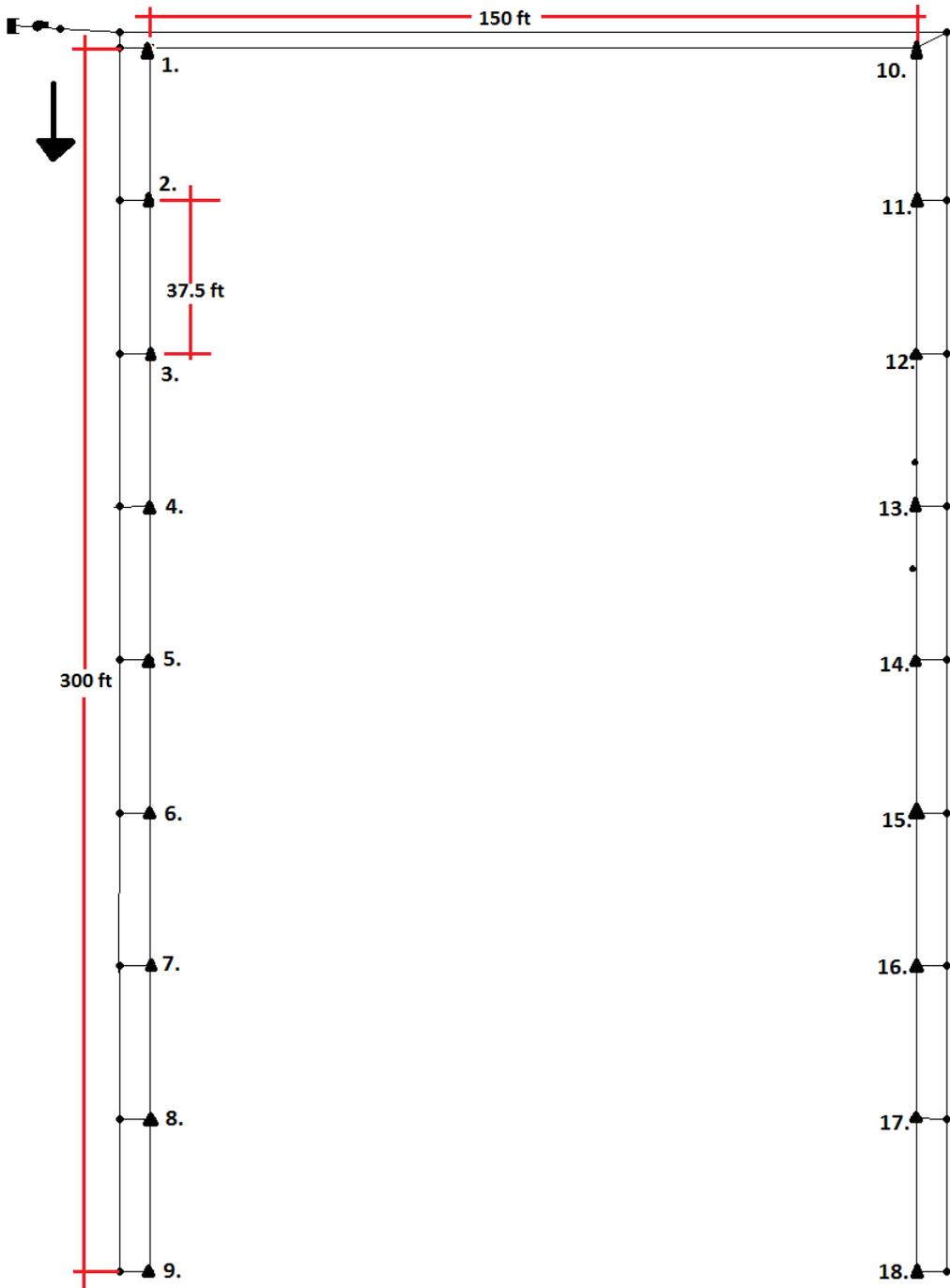
Figure 3 - Design 1: Exterior Loops. Triangles indicate sprinkler heads. Circles indicate connectors.
