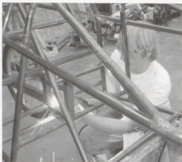
Junior Cory Pochop welds the rear drive terrain for the tech class's energy-powered electric car.
