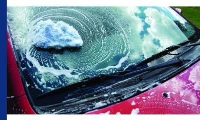
While you're at it, clean your wiper blades with a paper towel dipped in windshield washer fluid. This removes grime and oxidized rubber from the edge of the blade and helps prevent streaking. If streaks persist, you need new blade refills available from any auto parts store or discount chain.
