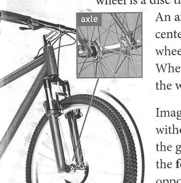
An axle is a rod. It is at the center of a wheel. It connects the wheel to a vehicle, like a bike.
