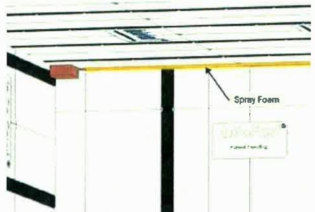
Spray foam the gap between ceiling and walls
