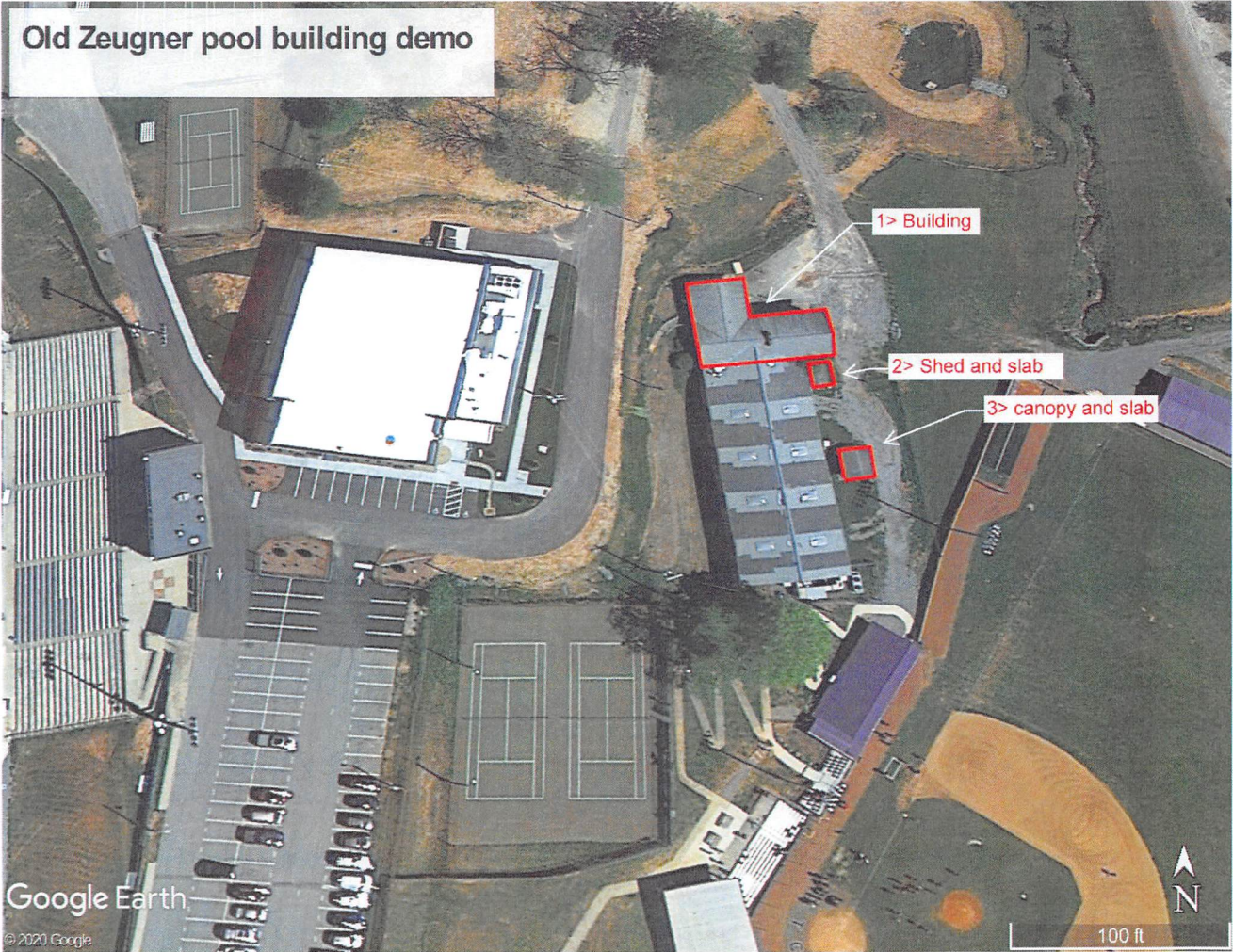
Buildings outlined in red to be demoed and removed. (including slab and foundation)
