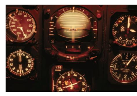
Figure 4 The speedometers and compasses on an airplane instrument panel tell the pilot the airplane's velocity.
