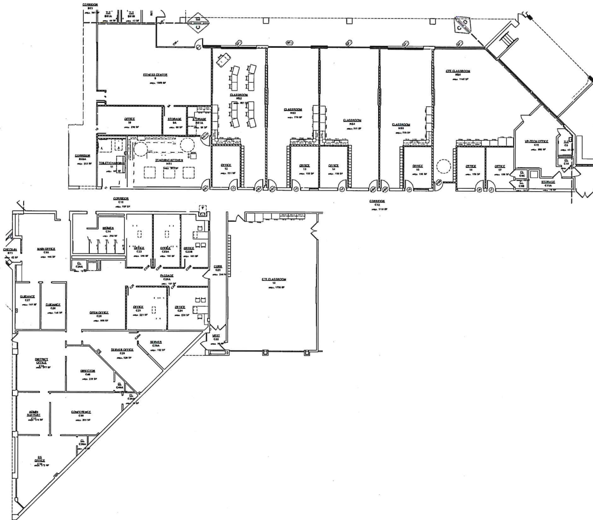
PLAN NOTATED FOR CLARITY PARTIAL DEMOLITION PLAN - FIRST FLOOR - AREA C SCALE: 1/8" = 1'-0"
