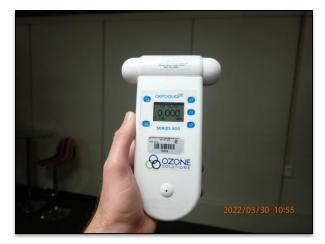
Figure (26) – Ozone meter measurement of 0 ppm collected from within Library.
