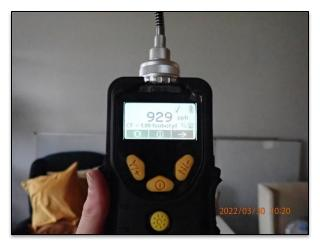
Figure (3) – PID Meter measurement of 929 parts per billion (ppb) room 7.
