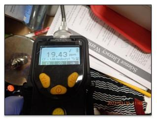
**Figure (5)** –PID Meter measurement within contents box with hand sanitizer 19.43 parts per million (ppm).
