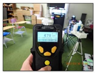
Figure (15) – PID Meter measurement of 478 ppb in Room 26.
