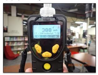
Figure (12) – PID Meter measurement of 388 parts per billion (ppb) library.
