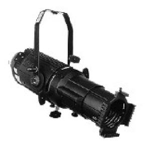
Altman Shakespeare S6-20 thru S6-50. A Standard Ellipses have three sets of lens chains. These are marked with 20°,30°, 40° and a 50° label on the lens barrel. This number related to the angle of the beam that emerges from the lens. These lights have a static lens chain. The lenses are seated in a tube that moves back and forth for focus. To change out the lens tube on an Ellipsoidal, unscrew the lens tube screw, and press the retaining clip in as the tube slides forward.
