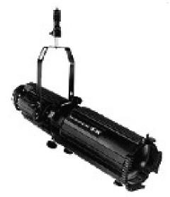
Altman Shakespeare S6-15-35 (Variable) A Variable is an ellipse where both lenses can be moved independently. There is no removable lens tube on a Variable. This type of light offers the most flexibility in the type of beam that it can throw. Variables are labeled
