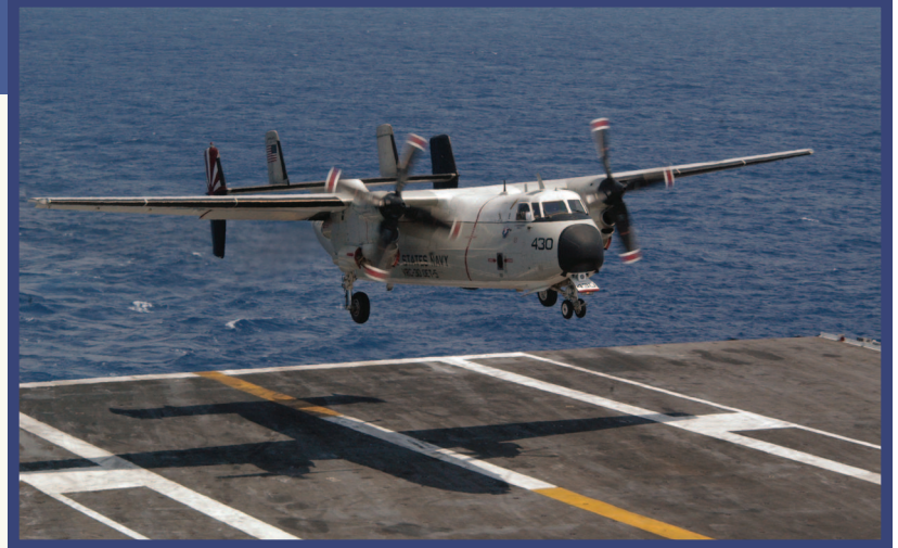
The primary mission of the C-2A Greyhound is carrier on-board delivery.
