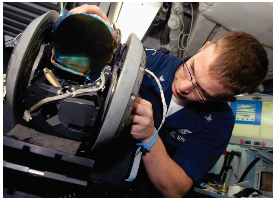
Aviation Electronics Technician 3rd Class Owen Snell rebuilds an advanced targeting forward looking infrared pod (AT FLIR), in the Advanced Intermediate Maintenance Division's Shop 4 aboard the nuclear-powered aircraft carrier USS Enterprise (CVN 65).
