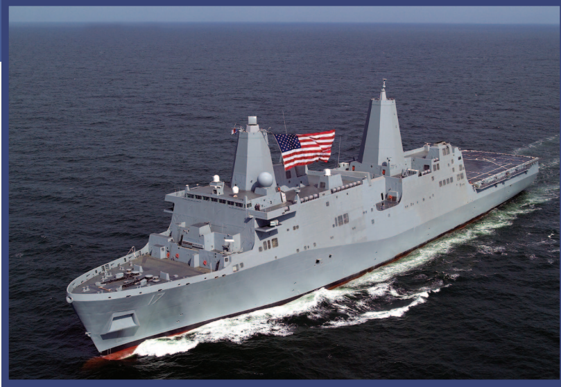
An amphibious transport dock like USS San Antonio can land troops by landing craft or helicopter.
