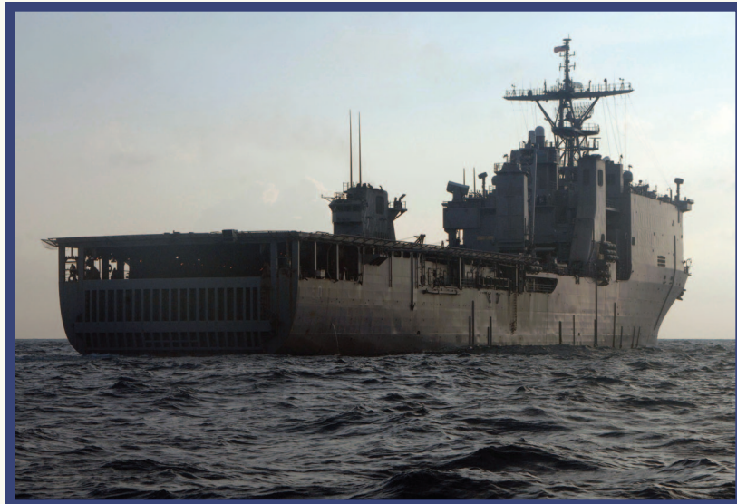
Dock landing ships such as USS Carter Hall carry and launch amphibious craft and vehicles as well as crew and troops.
