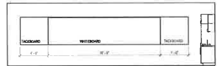
TYPICAL CLASSROOM ELEVATION - TEACHING WALL
