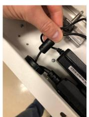
7. Plug iPad charger into the extension cord, pull iPad charge up through arm of the cart as shown. Then plug the iPad charger into the iPad.
