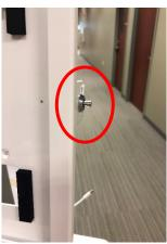
6. Place iPad in mount and shut the mount. Make sure camera is at the top of the ipad and the charger is at the bottom. To secure iPad in the mount press the pin in like shown.
