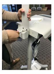
3. Remove the top of the JCO cart by loosening the 4 bolts underneath the edges of the JCO cart. There will be 2 on each side of the cart (do not remove the bolts completely). Take out accessory kit, this will be used for later.
